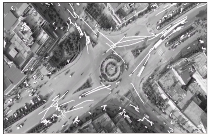
Fig 1: Shows the traced paths of objects detected in the video footage of a Nepali intersection. These traces are represented as white lines on the image. The traced paths provide information about the movement of the objects across the intersection, including their starting and ending points, and the direction in which they are moving.
