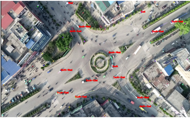
Fig: 2: Shows line traces of the detected vehicles in the Nepali intersection drone footage. The line traces represent the path taken by each vehicle, along with its origin and end direction.
